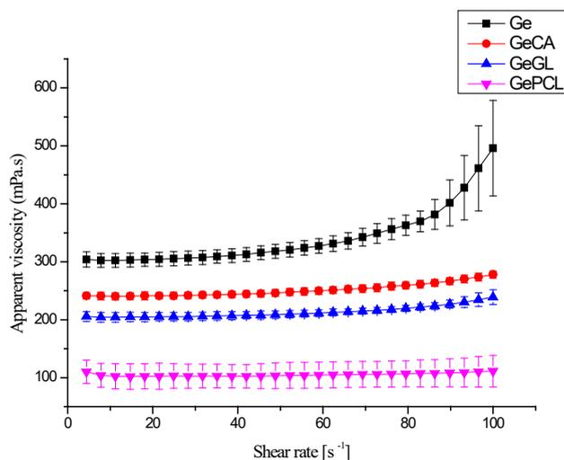
Figure 4. Flow curves of polymeric solutions: Ge, GeCA, GeGL and GePCL.
