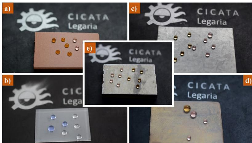
Figure 5. Photo of water droplets deposited on different substrates: a) quarry table tile, b) glass coverslip, c) galvanized steel sheet, d) copper sheet, and e) tile.
